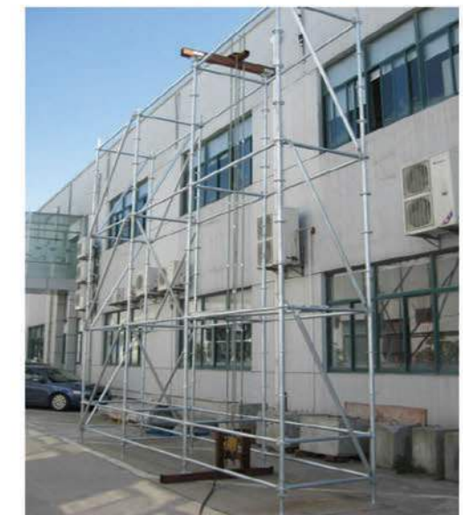
Ringlock Tower (One unit test)
