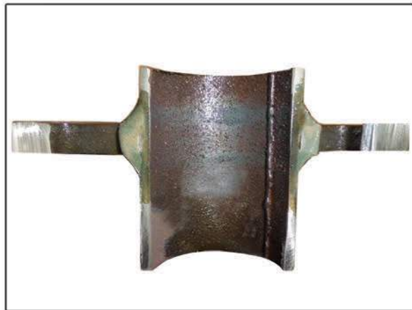
Rosette with tube welding
