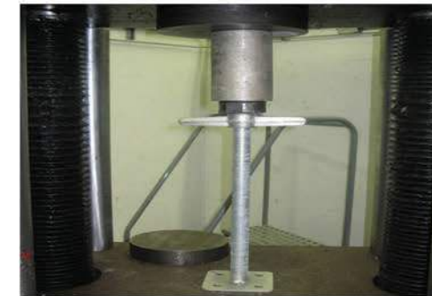
Base Jack (Test in different nut height)
