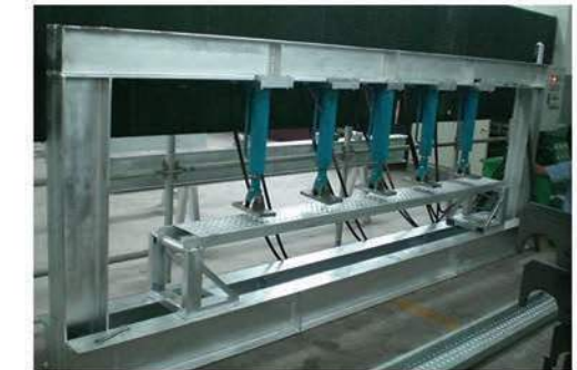
Steel Plank (Uniformly distributed load test)
