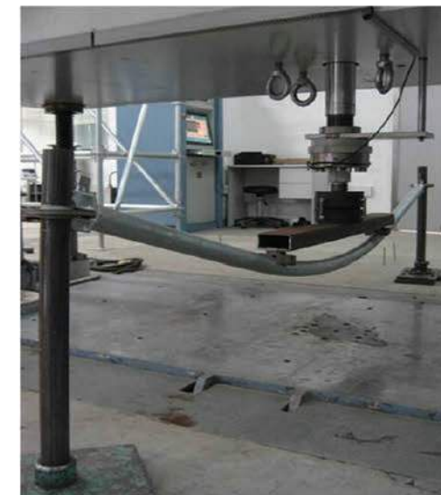
Ringlock Ledger (Load capacity test)
