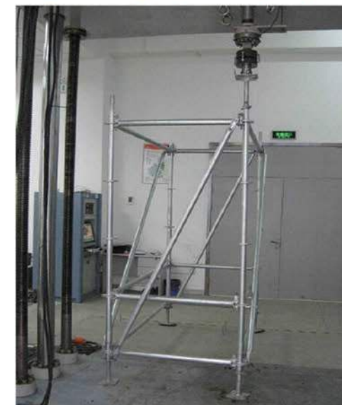
Ringlock Standard (Load capacity of single standard)
