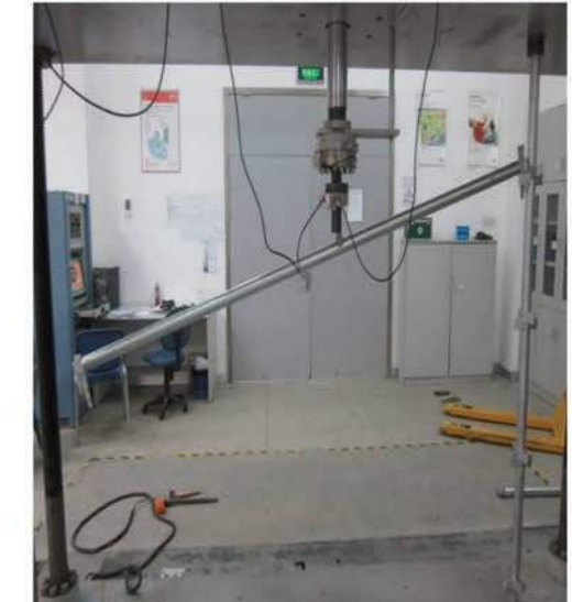
Kwikstage Ledger (Bending moment)
