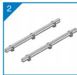
2 Fix the main beams
